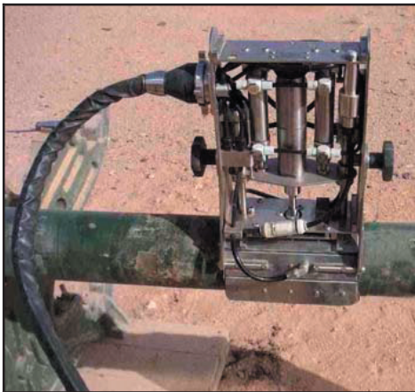
Seal insertion in an Iraqi 122mm rocket warhead suspected of containing nerve agent.
